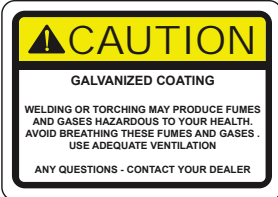
3) CAUTION: GALVANIZED COAT DECAL
