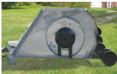
Smooth underdecks make for more efficient mowing and less area for rust to begin. Deck rings are standard.
